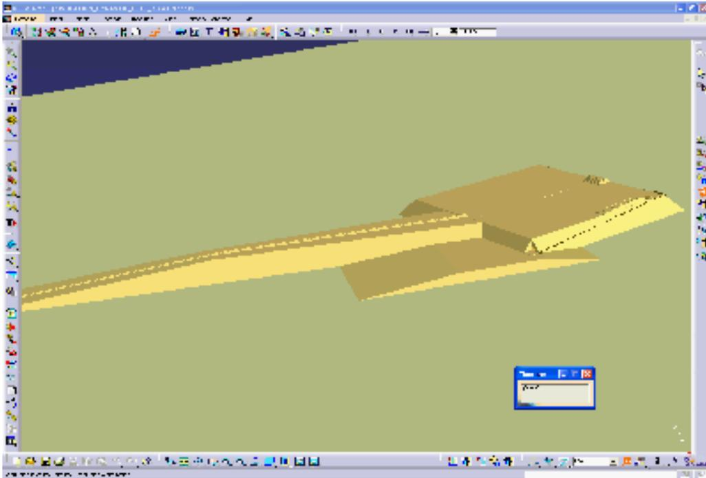
Integral simulation of the construction process in DELMIA: this software is also used to simulate the main stages of construction and visualise the logical sequencing of these stages by taking the time factor into account. This is the ninth year of the reign and the external ramp is providing a massive supply of stones of the right size to the site.
