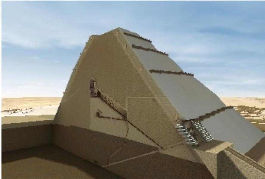
Nineteenth year of the reign, level +113 m is reached. North-South section as seen from the North East. Parts of the interior ramp can be seen embedded in the load-bearing masonry. The King's Chamber is now deeply buried in the mass of the monument. The cracks in the first ceiling have not yet appeared.
